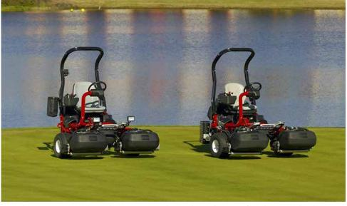
are the gas-powered TriFlex 3320 and diesel-powered TriFlex 3420. Both models feature an all-electric reel drive that reduce noise, eliminate hydraulic leaks and deliver plenty of power for unparalleled performance in challenging cutting applications. They include an energysaving mode that reduces the engine's RPMs while maintaining a constant reel speed through the all-electric reel drive. This results in lower fuel consumption and noise while maintaining quality of cut,
