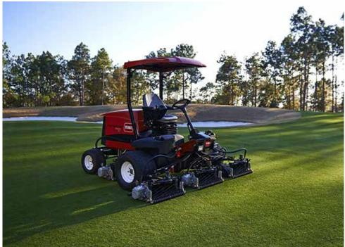
Triflex mowers. Like the eTriFlex 3370, the 3360's components for traction, steering, lift and cutting units are all-electric, and there are no hydraulics to leak.
