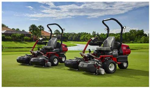
up to 35,000 square feet (over 3,000 square meters) of turf on a single charge. It features Toro's proven DPA cutting units and a 21-inch (53.34 cm) cutting width for a perfect combination of cutting performance, easy maneuverability and productivity. A convenient LCD screen gives the operator an instant view of the ongoing battery charge status and
