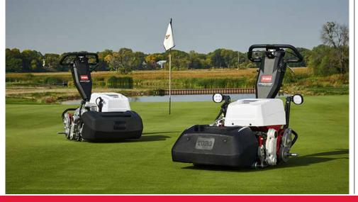
3370 operates with low noise. With greaseless bearings and no hydraulics to leak, the eTriFlex 3370 protects greens as well.
