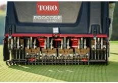
The ProCore 648s also delivers a faster return to playing conditions thanks to Delayed Mode. During operation, it continuously monitors the position of the coring head in its rotational path and the speed at which the coring head drops to ensure max tine depth on the first entries into the soil. In most turf conditions, this eliminates the need to repair tufted turf.
